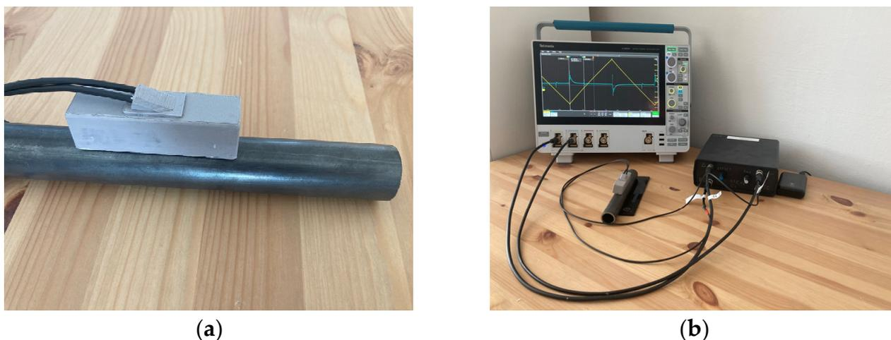
**Figure 16.** Experiment with a ferromagnetic core and external magnetic background. Figure (a) shows the coil system placed on the magnetic steel tube with a microwire inside. Part (b) shows the measurement under harsh conditions using analog RC filters. Part (b) also shows the measurement setup with the coil system, microwire (inside the magnetic steel tube), electronics, and Tektronix MSO44 oscilloscope.
