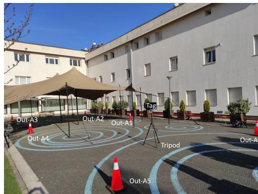
**Figure 8.** Set-up in the outdoor environment.
