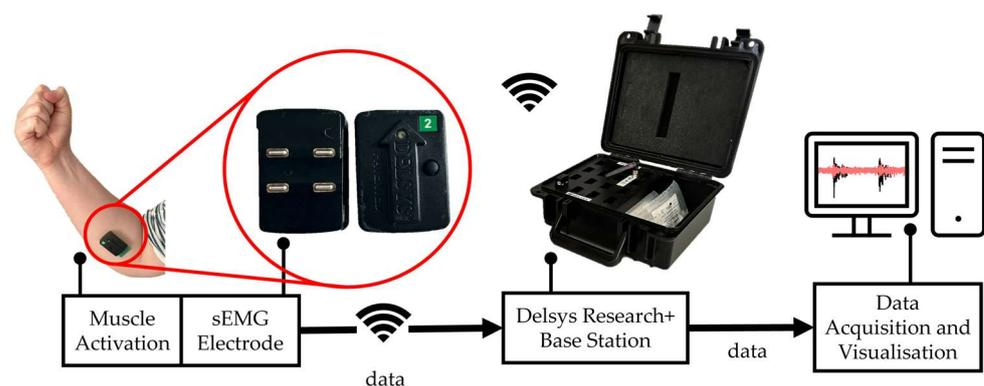
**Figure 2.** Block diagram of the measurement system illustrating steps involved in sEMG signal acquisition.
