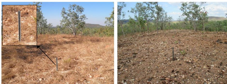
**Figure 2.** One of the erosion measurement locations showing the ‘V’-shaped dropper. The dropper extends 500 mm above the soil surface. The left photo shows conditions before burning while the right photo shows conditions following fire has been through the area. The surface displays a high rock content or armour.
