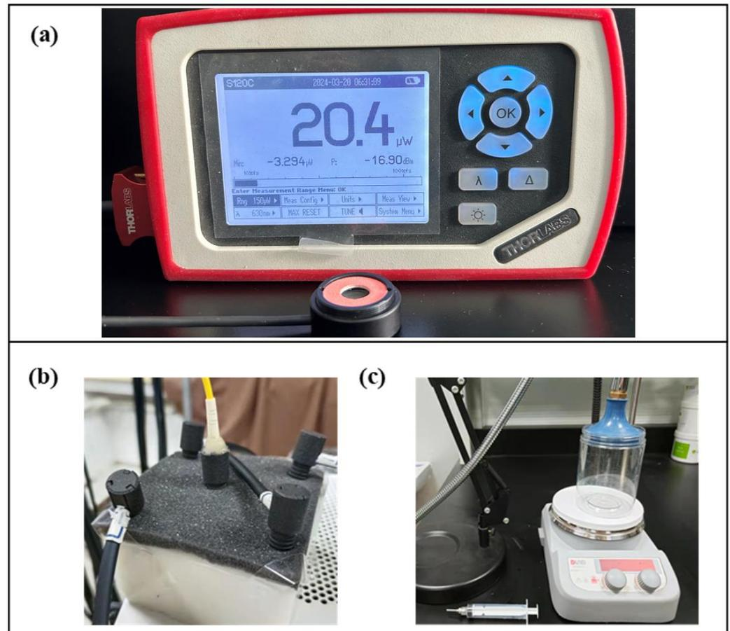
**Figure 3.** Experimental auxiliary equipment diagram. (a) The appearance of the luminous power meter. (b) A black sponge attaches a flexible probe to the optical phantom for evaluating stability, interference of background light, and inter-channel interference. (c) Blood model measurement system.
