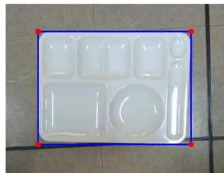
Figure 7. Finding four corner points of the meal plate for image transformation.
