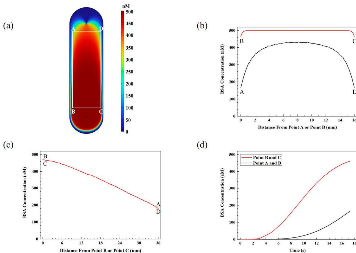
**Figure 2.** (a) Concentration distribution of BSA on the substrate surface after the injection of BSA at an equivalent volume of the large fluidic chamber; (b) concentration distribution of BSA along line AD and line BC in (a); (c) concentration distribution of BSA along line BA and line CD in (a); (d) the increase in BSA concentration over time at point A, B, C, D in (a) during BSA injection.
