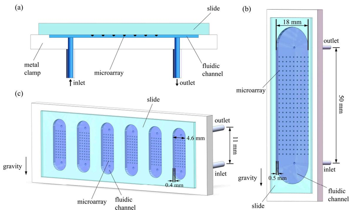
**Figure 1.** (a) Schematic of a flow cell, consisting of a metal clamp, a fluidic channel, and a glass slide with microarrays; (b) 3D representation of the flow cell with a large fluidic chamber; (c) 3D representation of the flow cell with six small fluidic chambers.
