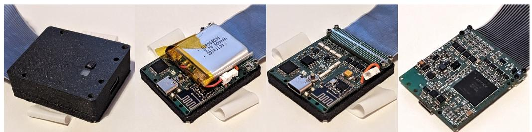
**Figure 10.** Readout module (left), readout board with a battery (2nd from left), without a battery and with a visible cable clamp (2nd from right), and the lower side of the readout board (right).
