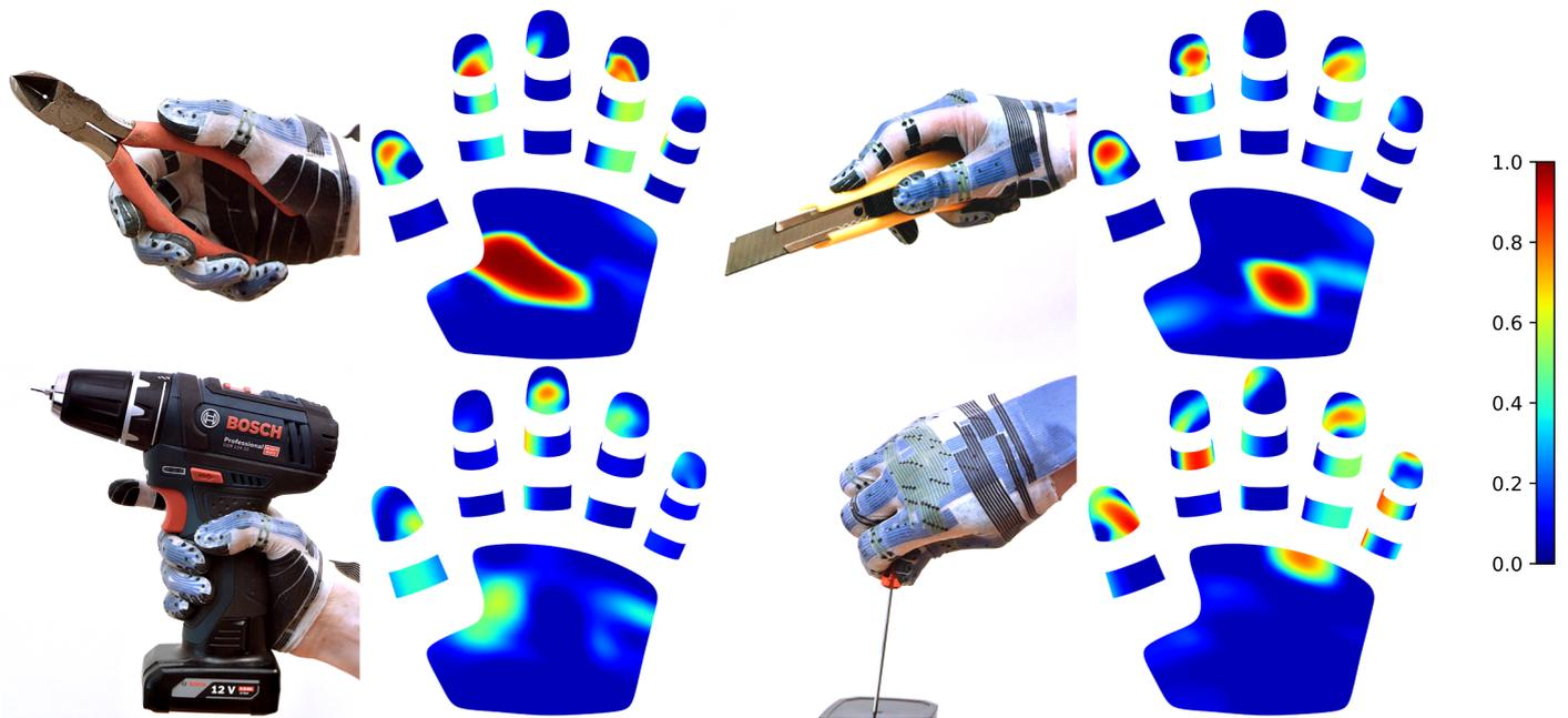
**Figure 14.** Manipulation experiments with a sensor glove prototype and corresponding tactile sensor readings. Sensor readings are visualized with a colormap (right) and a CAD model of the glove.
