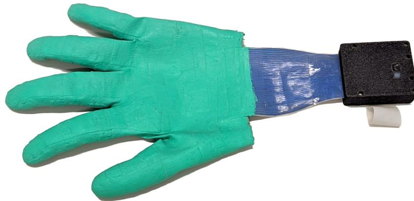
**Figure 9.** Fully assembled and painted sensor glove with readout module.
