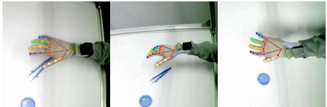
**Figure 11.** Multi-view false-color images of a sensor glove worn by a human and corresponding landmark detections from a neural hand-tracking network.
