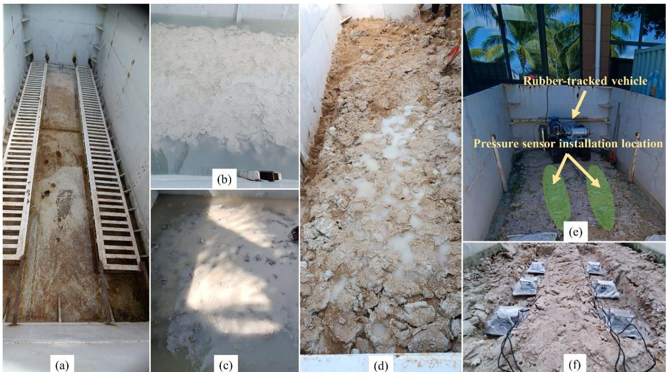
**Figure 5.** Experimental setup for Soil Bin and pressure sensor installation location: (a) Soil Bin used for the experiment, (b) Diatom soil in soil bin, (c) Bentonite soil in soil bin, (d) Sand gravel mixture mixed with bentonite soil, (e) Tracked vehicle and pressure sensor installation location, (f) front, mid, and Rear pressure sensor location in soil bin.
