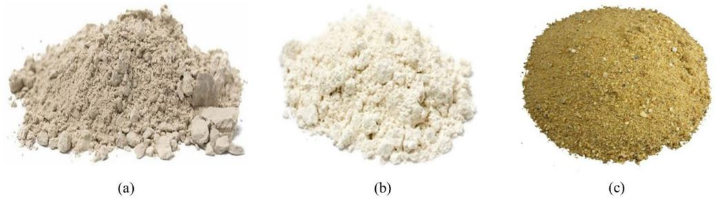
**Figure 10.** (a) Bentonite clay ( $-0.063$  mm), (b) Diatom soils ( $>20$   $\mu\text{m}$ ), and (c) Sand-gravel mixture (2~5 mm) were used in the experiment.
