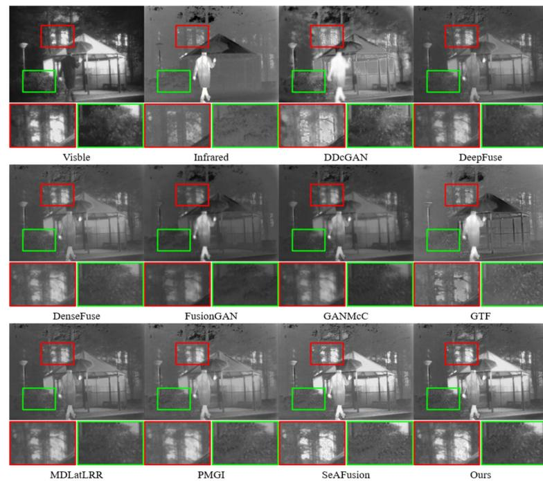
**Figure 8.** Qualitative comparison of the proposed method with nine SOTA methods on Kaptein 1654. For a more distinct comparison, a texture-rich area and a prominently targeted area (i.e., green box and red box) are outlined in each image.
