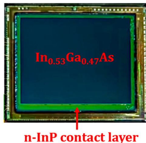
Figure 3. Top view of the InGaAs FPA after SiN passivation.
