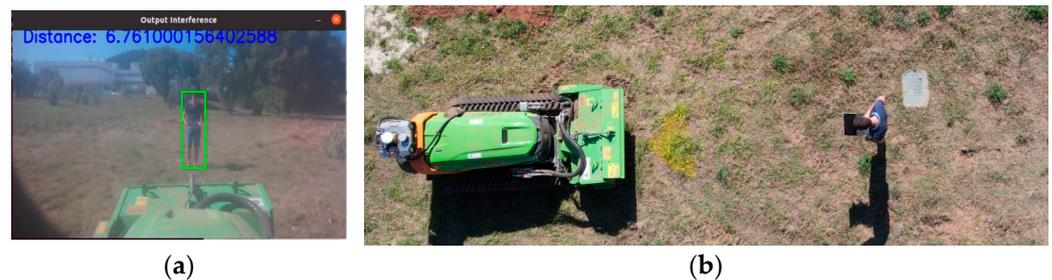
**Figure 9.** Test to verify the measurement from the camera. (a) Procedure for one of the stages of testing the vision system algorithm in the field. (b) The person located 6 m from the front camera of the Sentry.
