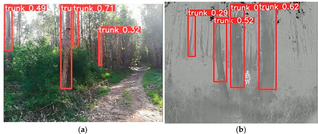
**Figure 11.** Images taken from the qualitative test regarding the *Trees\_dataset*. (a) Image taken by the RGBD camera; (b) image taken by the thermal camera.
