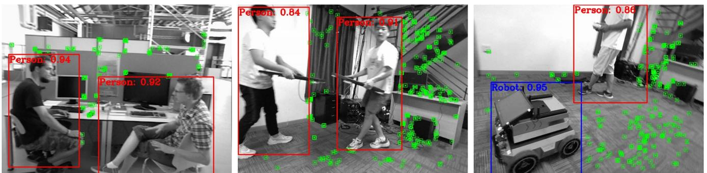
**Figure 9.** The feature extraction effects of GY-SLAM on different datasets. The green boxes represent the ORB feature points extracted by the SLAM system.
