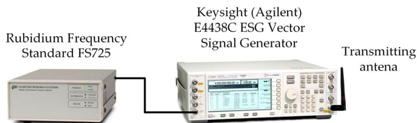
**Figure 2.** Transmitting part of test-bed for frequency stability measurement.
