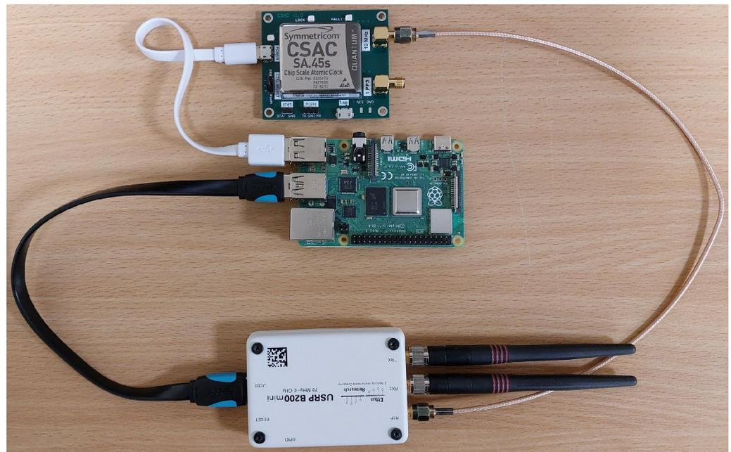
**Figure 14.** Hardware structure for a location sensor consisting of SA.45s CSAC, Raspberry Pi 4 model B, and USRP B200mini-i.
