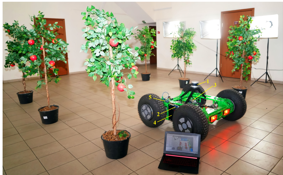
Figure 3. Conducting an experiment in a laboratory based on a robotic platform with a motion control system based on laser location methods: 1—LiDAR Velodyne Puck (VLP-16); 2—top-level control system unit; 3—BM1418ZXF DC motor; 4—Benewake TFmini Plus rangefinder; 5—system unit lower-level controls.
