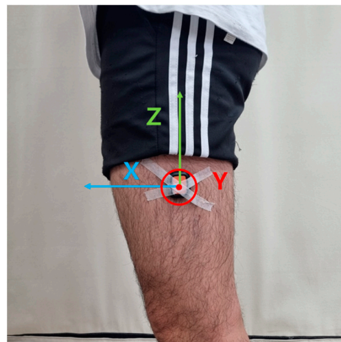
Figure 1. The IMU sensor orientation. X axis: anterior–posterior direction, Y axis: medial–lateral direction, and Z axis: superior–inferior direction.
