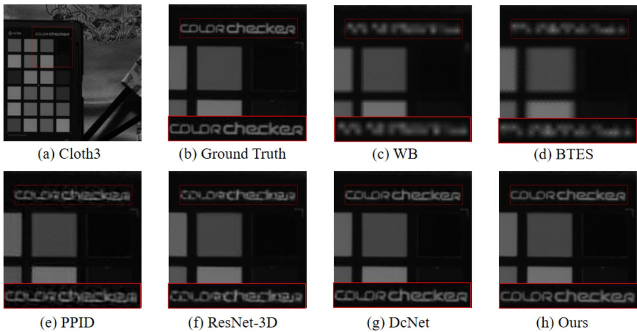
**Figure 7.** The visual quality comparison results of different demosaicing methods for cloth3 scenes. (a,b) is the reference image and the ground truth. (c) is the result of the WB. (d) is the result of the BTES. (e) is the result of the PPID. (f) is the result of the ResNet-3D. (g) is the result of the DcNet. (h) is the result of ours.
