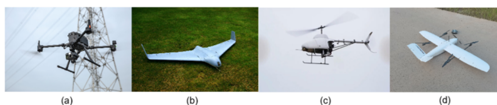
Figure 10. Different UAV platforms: (a) Multi-rotor UAV, (b) fixed-wing UAV, (c) unmanned Helicopter, and (d) VTOL UAV, obtained from Zhang et al. [90].
