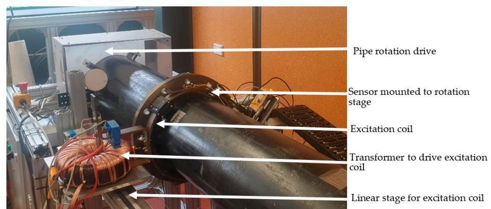
**Figure 11.** Photo of experimental setup with coil encircling pipe.
