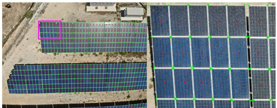
**Figure 4.** Detection results. On the (left), full image of  $1024 \times 1376$  provided to the detector. On the (right), a zoom in of the magenta bounding box. Object center detections are depicted with red dots, while the green dots depict the detected keypoints per object.
