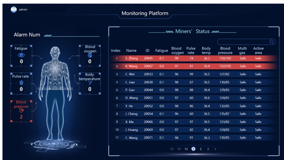
Figure 11. Interface of monitoring platform for miners' status.
