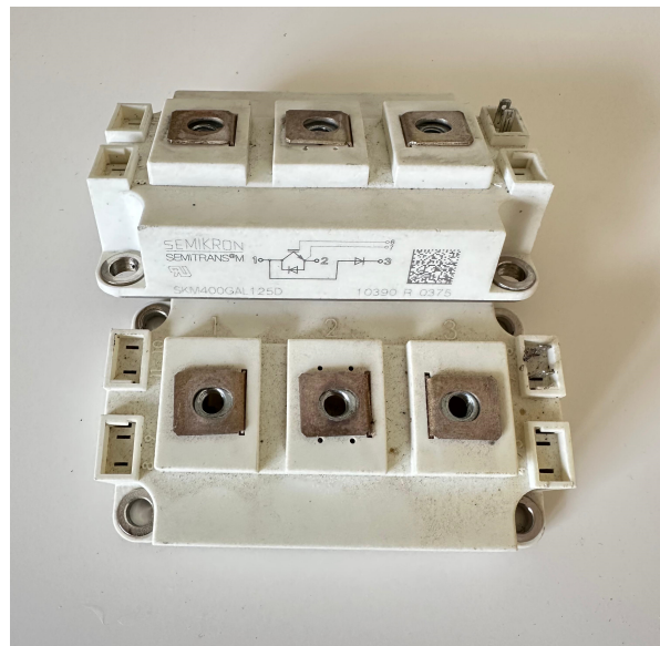
Figure 6. Transistors IGBT SKM400 with high current terminals.
