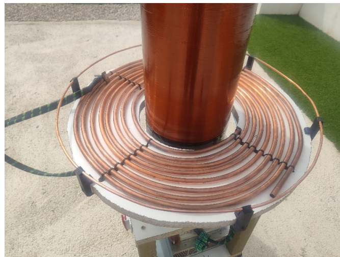
Figure 5. Primary resonant circuit based on a flat concentric copper tube and secondary resonant circuit with vertical coil.
