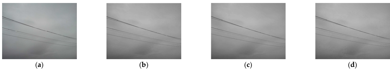
Figure 10. Image grayscale effect processing diagram. (a) Original image; (b) Average method; (c) Weighted average; (d) Maximum value method.
