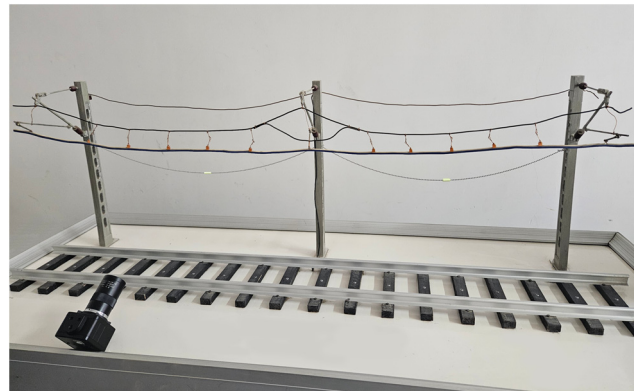
Figure 21. Video monitoring simulation test platform for OCS additional conductor oscillation.
