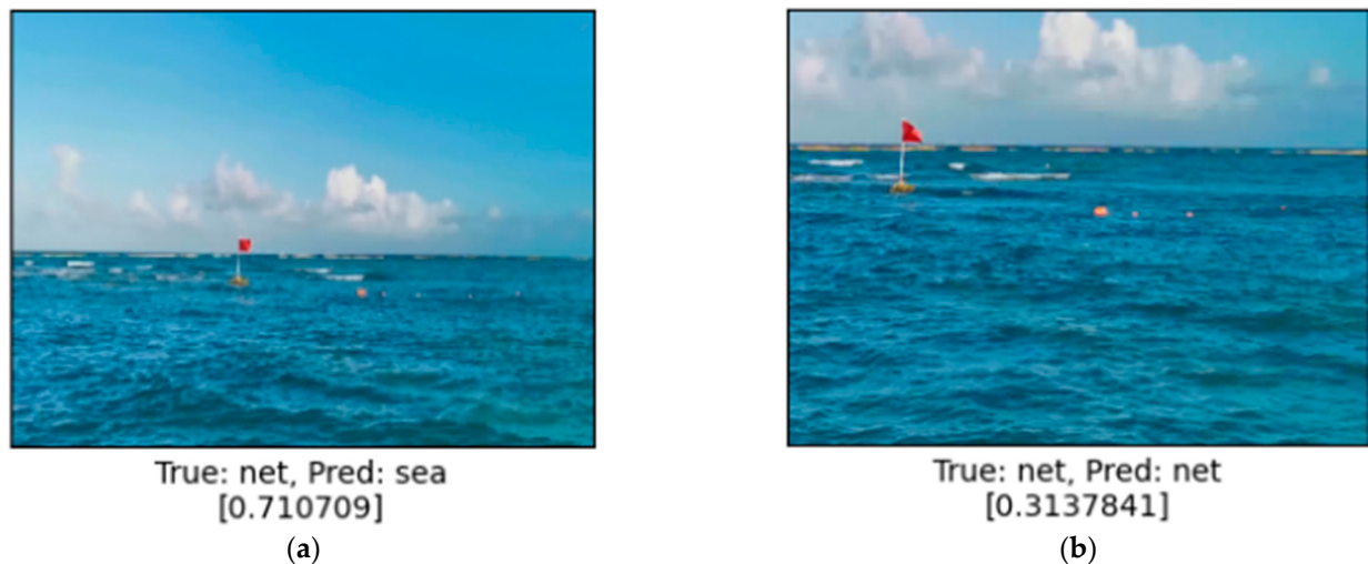
Figure 8. Comparison of network results depending on distance to floating objects. Range of values is a real value from 0 (not safe) to 1 (safe). Safety level in square brackets. Longer distance (a) qualifies situation as relatively safe (0.71). When vessel approaches a little closer (b) then safety level drops significantly to 0.31.
