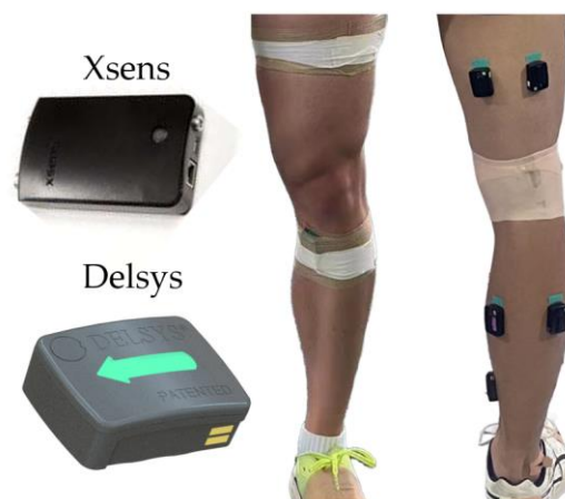
Figure 2. Wearing position of inertial measurement unit and electromyography sensor.
