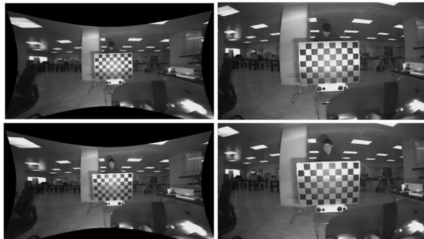
**Figure 23.** Aberration and correction maps for visible light camera (left lens).
