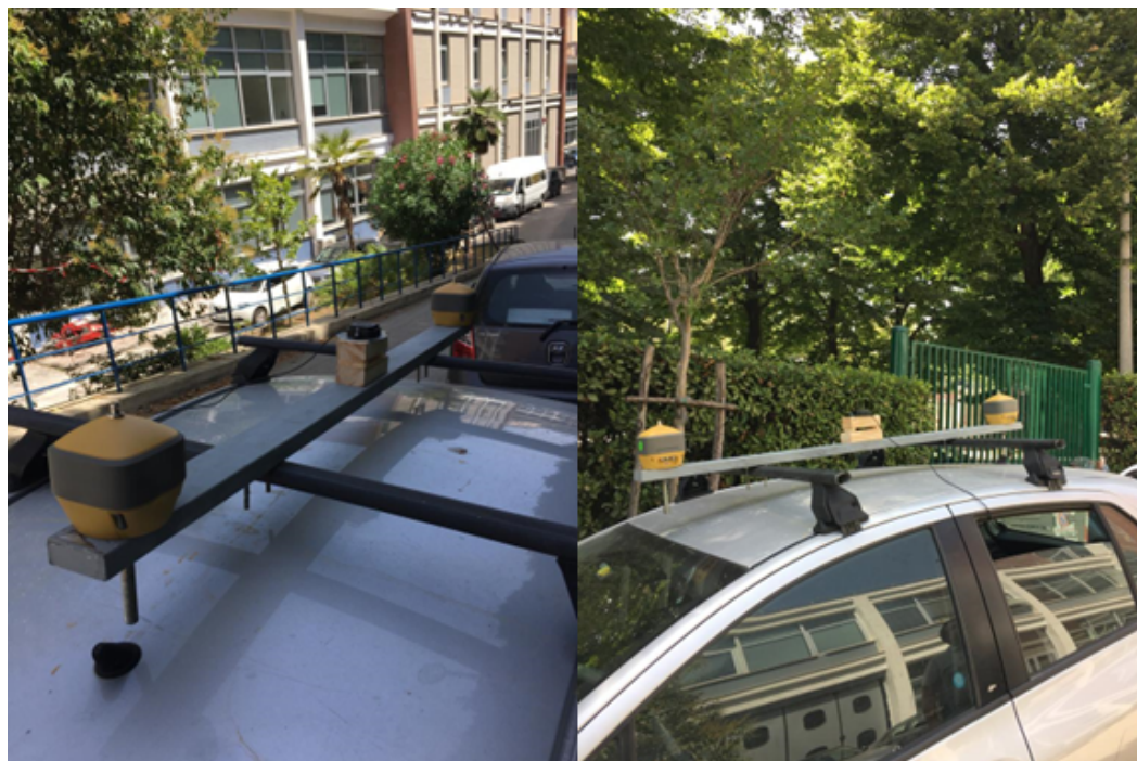
Figure 7. Images depicting the bar mounted on the test car. The left image displays a frontal view, while right image displays a side view. It is worth noting that a wood base of a certain thickness was employed to align the phase centres of the three antennas.
