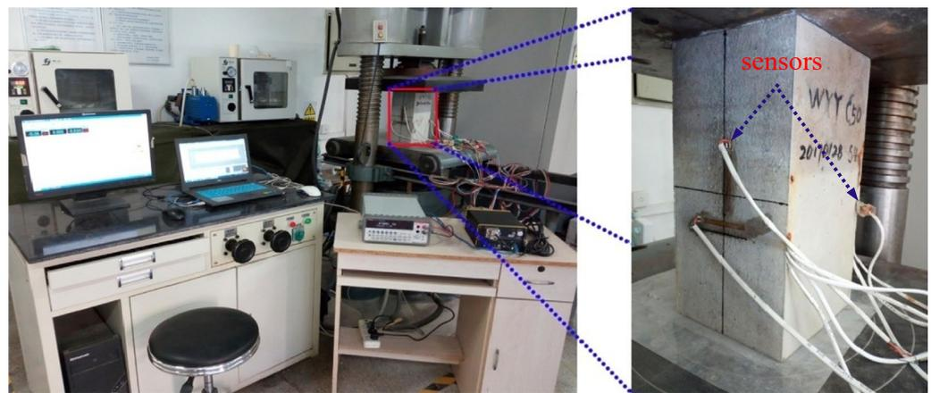
**Figure 5.** The sensors and experimental platform for monitoring of concrete structures [75]. Copyright 2019, Elsevier.
