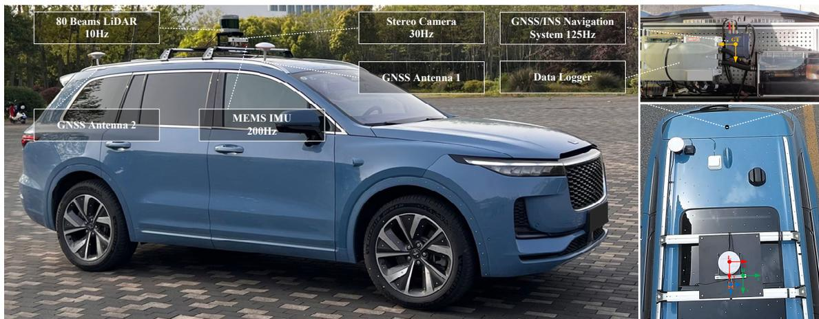
**Figure 13.** The data collection vehicle and equipped sensors.
