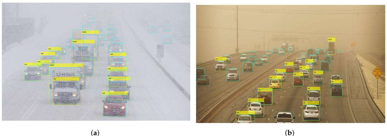
**Figure 14.** Missed vehicle from YOLOx in bad weather, (a) snow, and (b) sandstorm.
