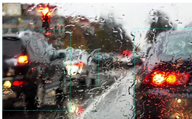
**Figure 17.** No detection in screen covered by rainwater.
