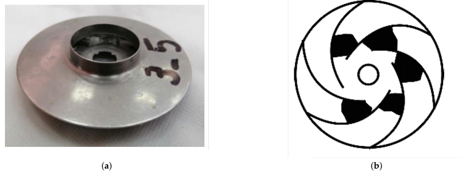
Figure A5. An example of impeller channel blockage is shown. The levels of blockage severity are attained by closing different channels of the impeller. (a) Appearance of the impeller channel blockage. (b) Drawing representing the impeller channel blockage.
