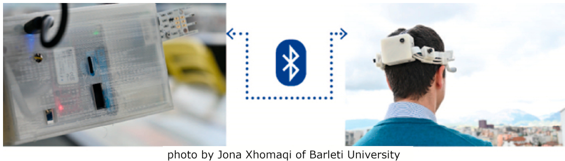
Figure 3. Fully wearable system with a detail of WEMOS (Wearable Environmental Monitoring System) used during the test experiment.
