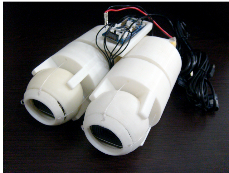
Figure 6. Tendon-driven, 3D printed robotic model of the human eye (robotic eye). The details of the interior structure of the robotic eye, including its design and functionality, are thoroughly discussed in [14].
