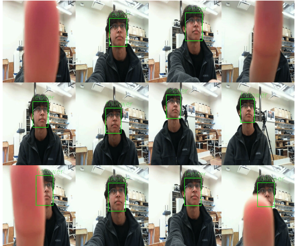
Figure 5. An instance of the face tracking running on the robotic eye, with the tracked face highlighted by a green bounding box. The experiment involved the test subject moving before the eyes and crossing the corners of the image at six different locations, with full and partial occlusion occurring in the first and last rows of the figures, respectively.
