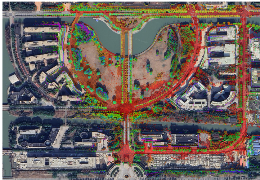
Figure 5. Mapping result of BA-CLM aligned with Google earth on M2DGR dataset [33].
