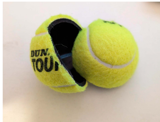
Figure 1. Cutting open a hollow-body pressurized tennis ball shows a layer of rubber inside the layer of felt. Reassembling the open ball will cause inconsistent surfaces, causing inconsistent rebounds.
