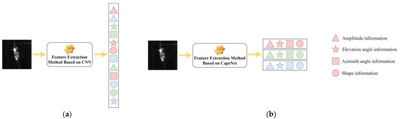
Figure 4. Comparison of two feature extraction methods. (a) Feature extraction method based on CNN; (b) Feature extraction method based on CapsNet.
