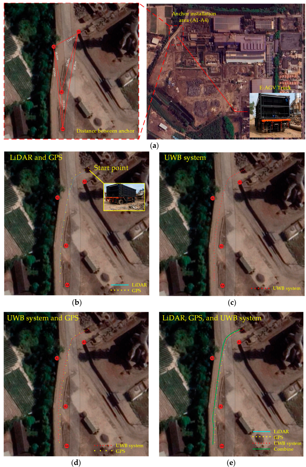
Figure 11. Testing autonomous electric trucks in real factory locations in conditions using different sensors for navigation: (a) installing anchors (A1–A4) in narrow road areas in factories; (b) GPS and LiDAR; (c) UWB sensor; (d) GPS and UWB sensors; and (e) LiDAR, GPS, and UWB sensors.
