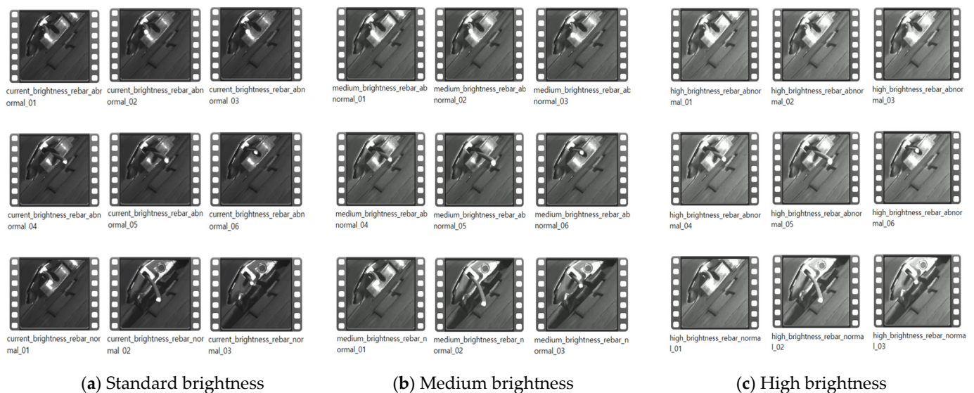
Figure 4. 27 videos of the rebar extrusion process under different lighting conditions: (a) standard brightness (brightness level ~64,200 W LED, 10 ms exposure); (b) medium brightness (brightness level ~96,200 W LED, 15 ms exposure); (c) high brightness (brightness level ~128,200 W LED, 20 ms exposure). Each row within a lighting condition shows abnormal ( top and middle ) and normal ( bottom ) rebar extrusion processes.
