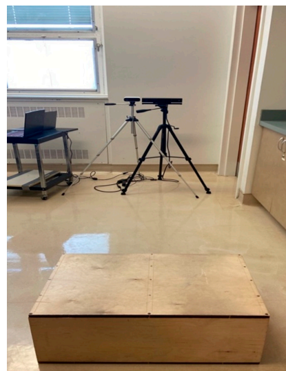
Figure 2. Image displaying the Azure Kinect and Kinect V2 mounted on tripods at a distance of 2.5 m from a 31 cm box for optimal accuracy.
