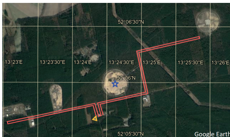
Figure 2. Satellite image of blast test site where the fiber-under-test (FUT) is represented by a line (red), the location of the blasts by a star (blue) and the \phi_g -OTDR test setup by a triangle (orange) pointing to the beginning of the FUT to which it is connected.
