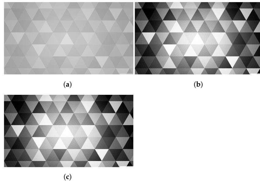
**Figure 11.** (a) Figure before histogram equalization. (b) Figure after histogram equalization with FPGAs. (c) OpenCV histogram equalization output image.
