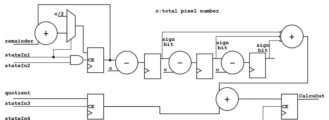
**Figure 9.** The architecture of the integrator.
