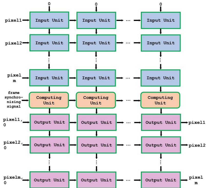
Figure 1. Two-dimensional configurable pipeline architecture.
