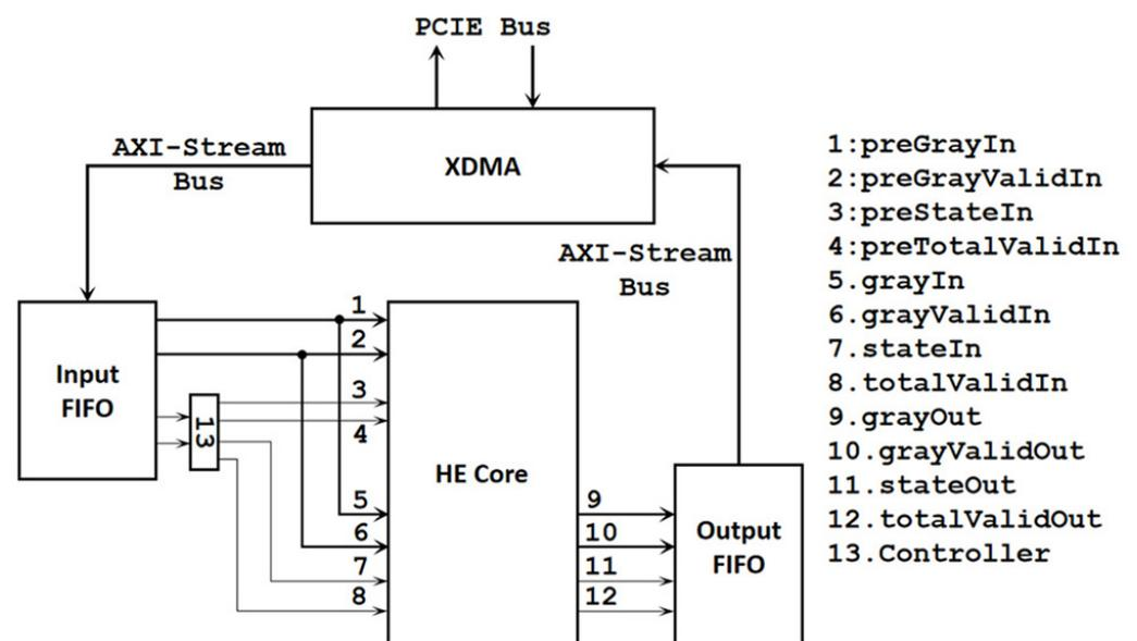
**Figure 3.** Overall architecture utilizing only CL.
