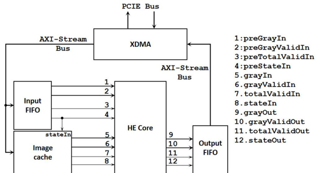
Figure 10. Overall architecture utilizing CL, DSP, and BRAM.
