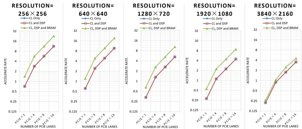
**Figure 15.** Acceleration rate for a single-core CPU.
