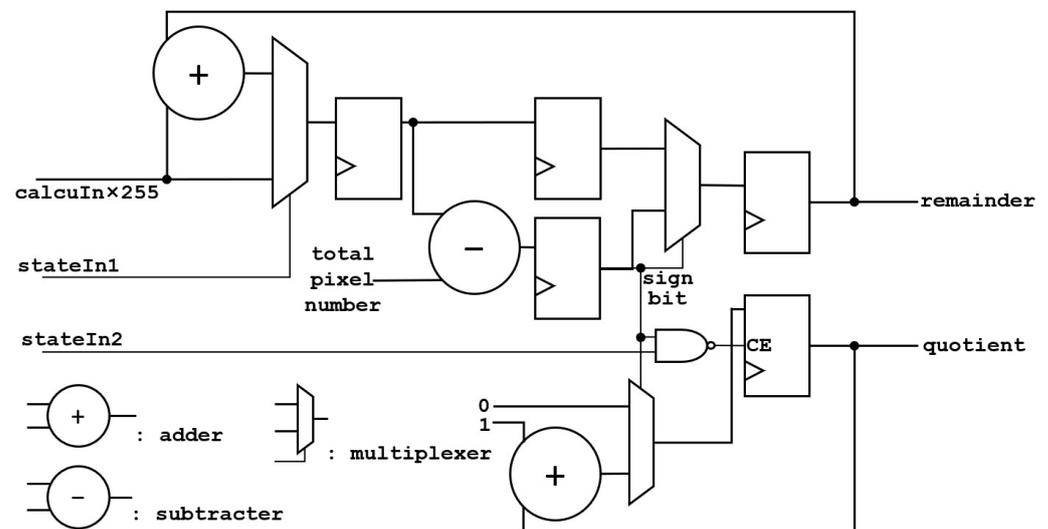
**Figure 8.** The architecture of the accumulator.
