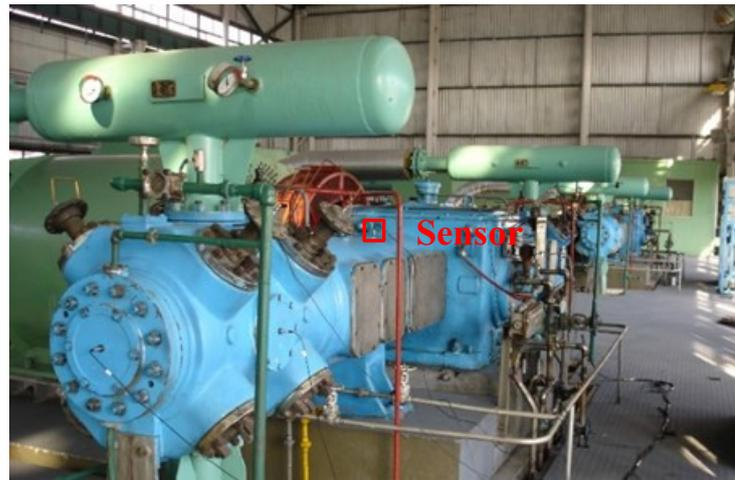
**Figure 26.** DW-10/12-27-XIII type two-stage double-acting reciprocating compressor.
