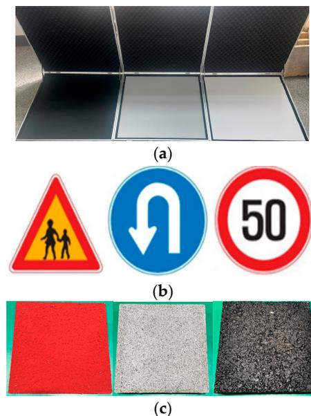
**Figure 2.** Materials employed for testing. (a) Reference Materials (RM 5%, 50%, 95%); (b) Traffic signs (school zone, U-turn, speed limit); (c) Pavement materials (skid resistance, concrete, asphalt).
