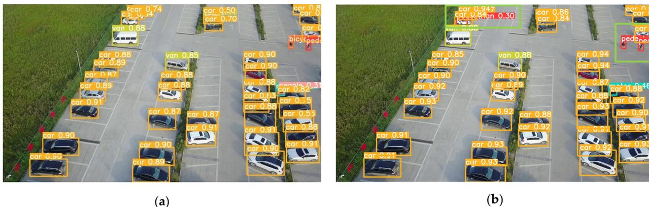
Figure 9. YOLOv5s vs. SMT-YOLOv5: dense distribution detection. (a) result of YOLOv5; (b) result of SMT-YOLOv5.
