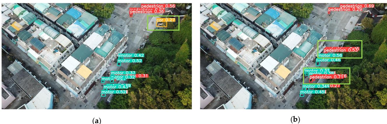
Figure 10. YOLOv5s vs. SMT-YOLOv5: complex background detection. (a) result of YOLOv5; (b) result of SMT-YOLOv5.
