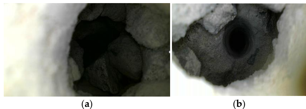
Figure 16. Drilling verification results photos. (a) The endoscopic photograph at 5 m; (b) the endoscopic photograph at 43 m.
