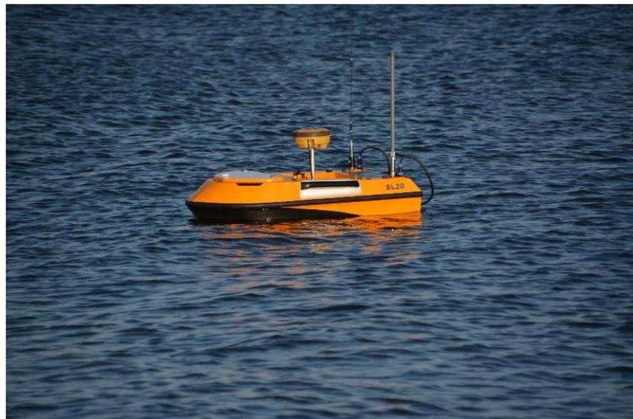
**Figure 4.** USV OceanAlfa SL20 during bathymetric survey.
