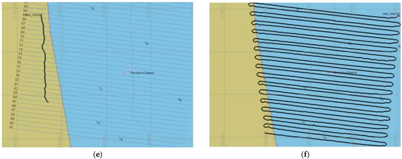
**Figure 2.** Stages of planning the survey lines in the restricted area: (a,e) rectangular area including shallow water and land area, (c) area limited using the ENC, (b,d,f) trajectory of the USV on reduced survey lines.
