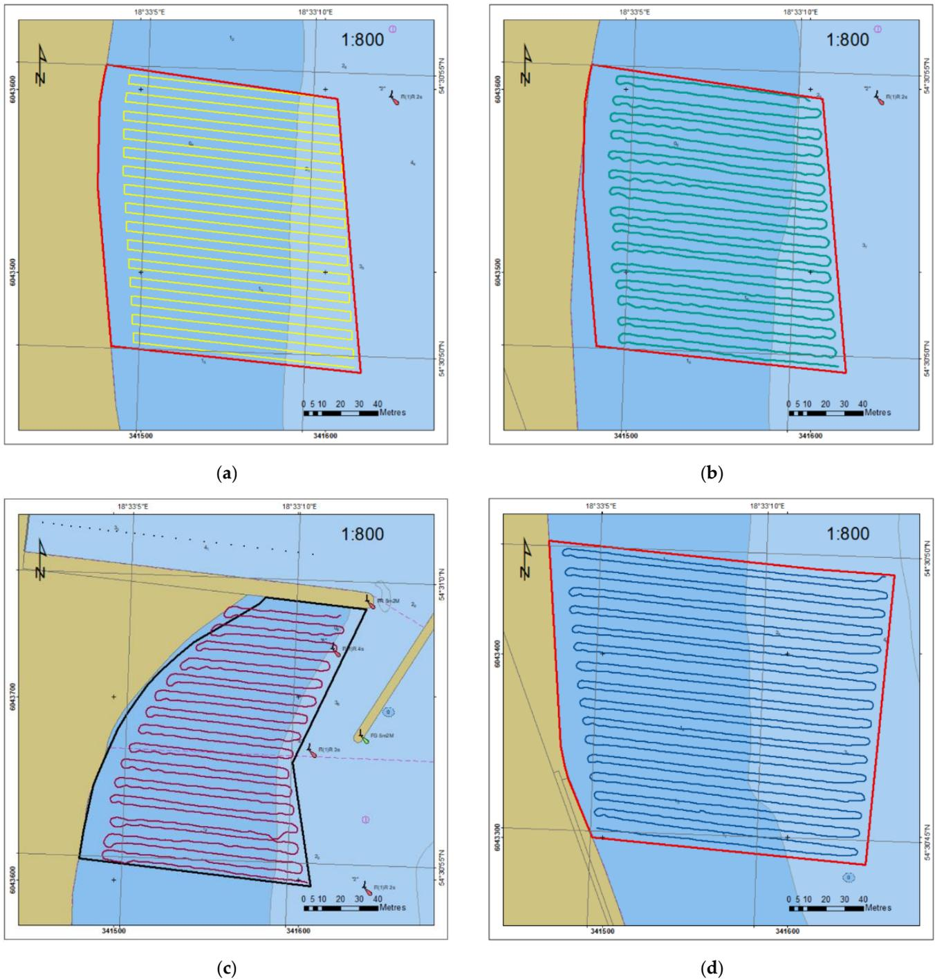
**Figure 6.** Planned lines in area B (a) and the trajectory of the USV in restricted areas: B (b), A (c) and C (d).
