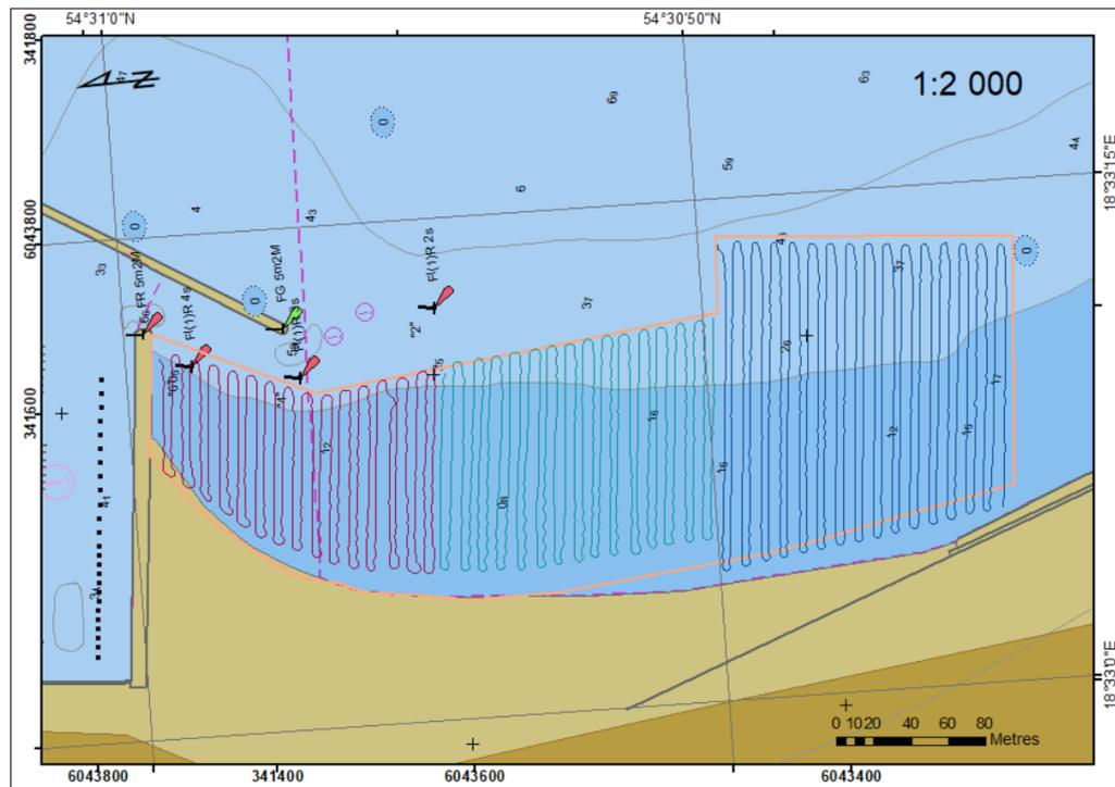
Figure 7. Sounding region with the USV's trajectory.
