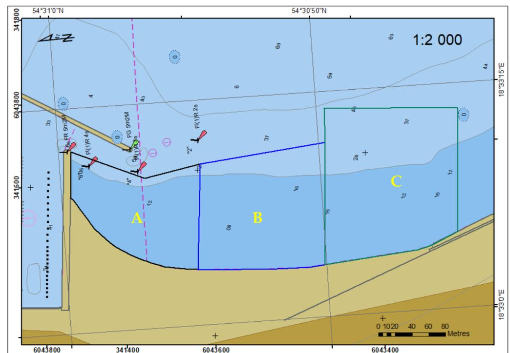
**Figure 5.** Sounding area divided into three parts.
