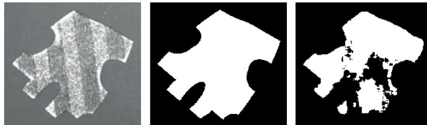
**Figure 14.** Segmentation error of part 4 at height 25.2 mm due to inhomogeneous lighting. Left: Camera image, middle: mask, right: segmentation.
