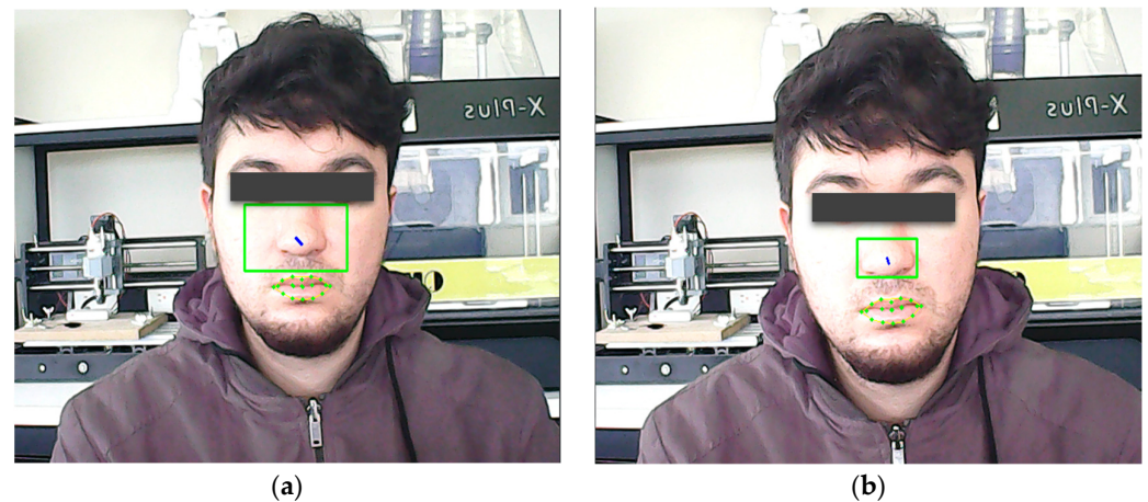
Figure 7. Green boundary box size comparison. (a) Rectangle of size 65 \times 35 pixels/frame processed; (b) rectangle of size 35 \times 20 pixels/frame processed.
