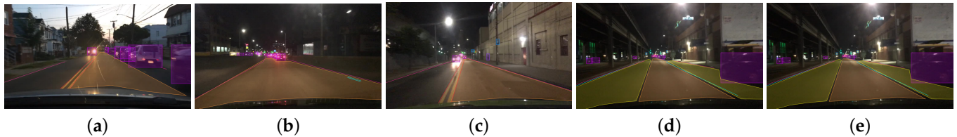
Figure 16. Visualization results of ANU tracking system on BDD100K data set. (a) shows the results of vehicle detection and tracking during the day, (b–e) show the results of vehicle detection and tracking at different times of the night for the same video.
