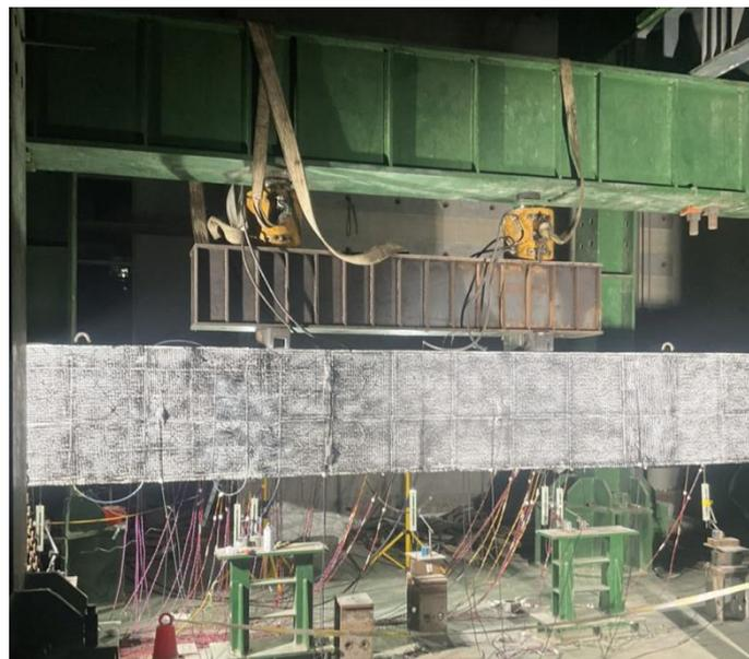
**Figure 2.** Laboratory test setup of precast segmental bent cap.
